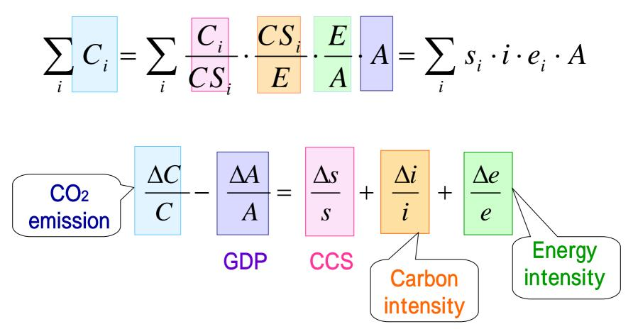
CO<sub>2</sub> emission is reduced by combining introduction of CCS, decrease of carbon intensity and improvement of energy intensity.
