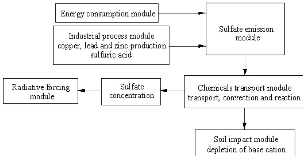
Figure E-8-1 Framework of sulfur emission and deposition model.
