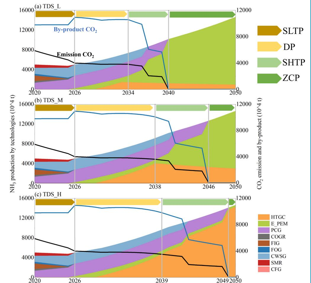
**Fig.1 The ammonia industry zero carbon pathways, CO<sub>2</sub> emissions and by-product CO<sub>2</sub> generation under different scenarios.**
