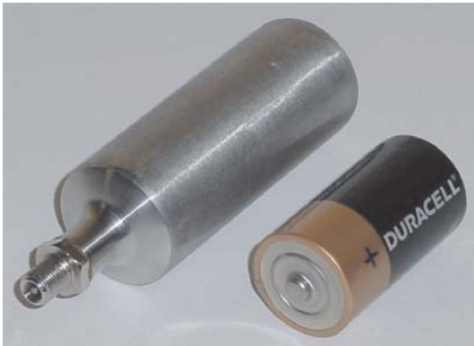
Figure 1. 20 l of hydrogen storing metal hydride container and a normal D-type battery.
