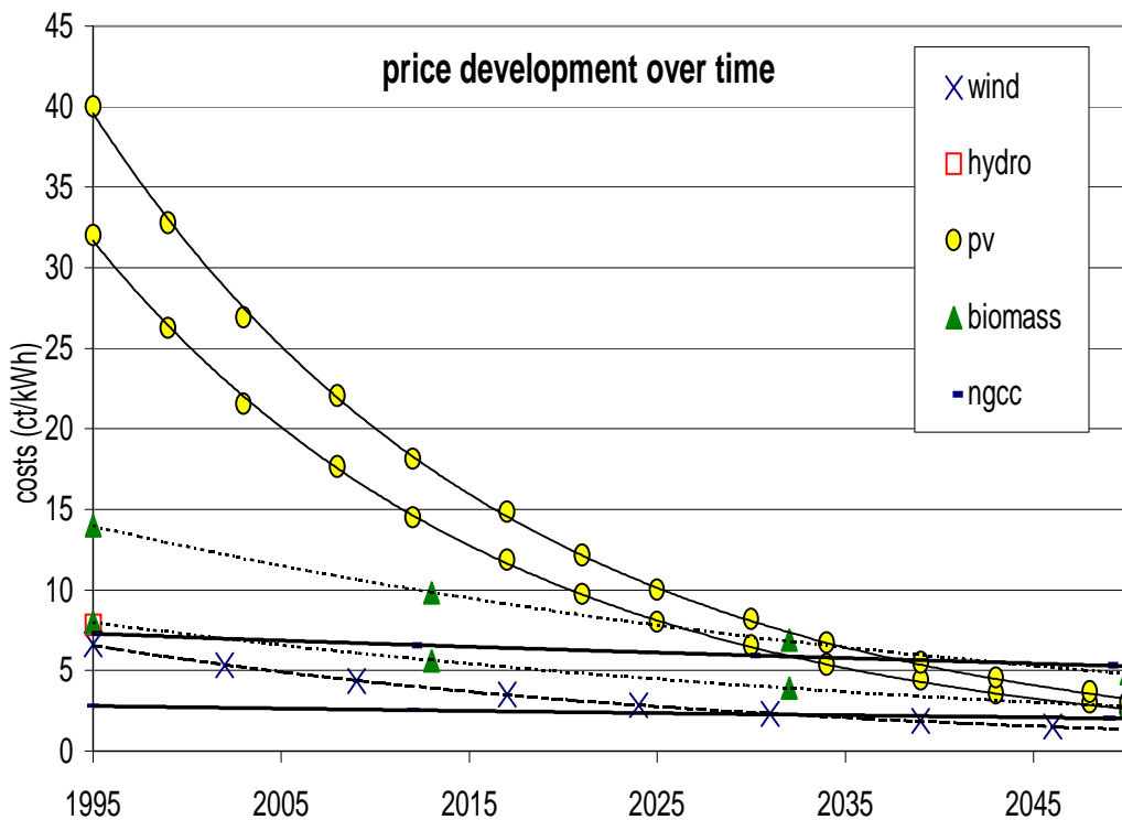
Figure 1.4. The development of electricity costs by source over time ($ct/kWh). For the gas-fired plants (NGCC) the high estimate reflects a plant with CO 2 removal and storage, while the lower figure does not include the removal and storage option. In the current image no CO 2 removal and storage is assumed.
