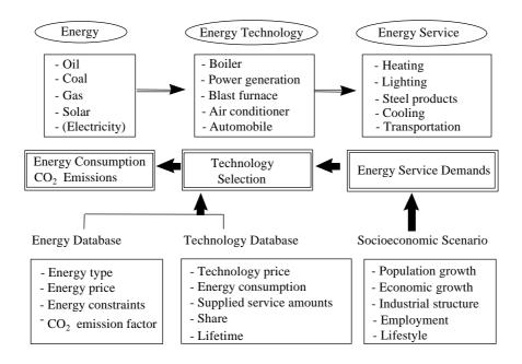
Figure 1 Structure of the AIM/end-use model
